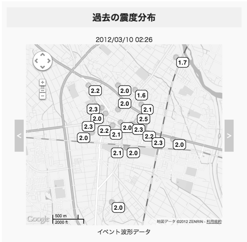
Figure 7: On-line viewer system displaying the distribution of seismic intensities at the array. The locations correspond to the station locations in Fig.3.
